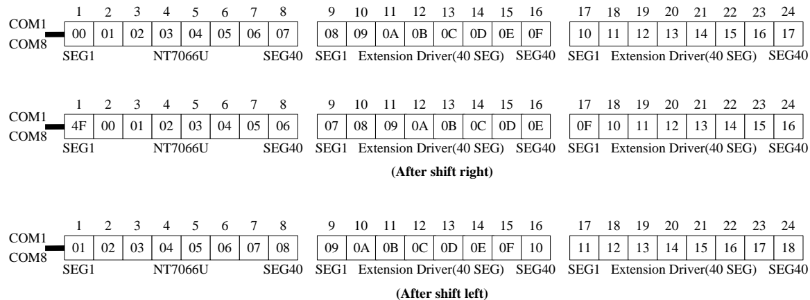
Fig.2. 1-line X 24ch, display with 40 SEG & extension driver.
